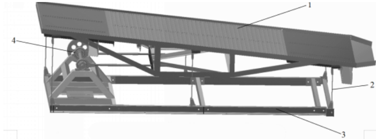
Figure 3. 3D model drawing of the vibration motor; 1: frame; 2: spring plate; 3: base; 4: transmission parts
