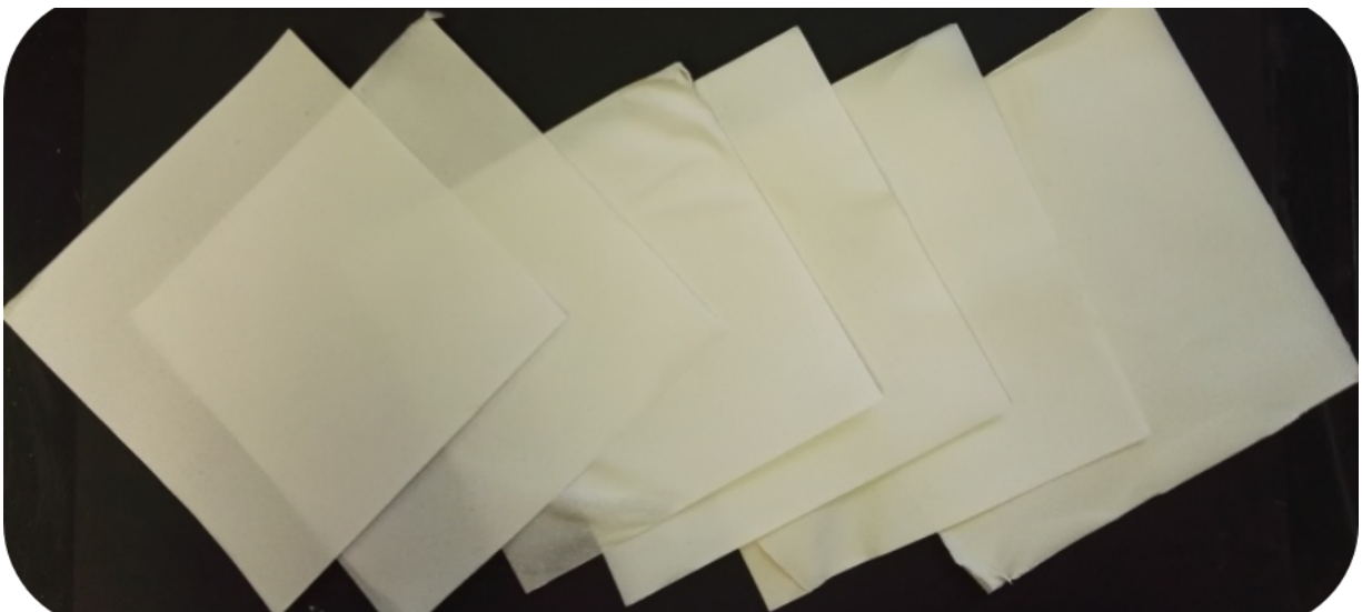
Figure 1. Spray-coated nanocomposites prepared via spraying cellulose nanofiber; MMT produced from spraying of CNF; Closite Na ++ suspension on the stainless-steel plate. The size of cellulose nanofiber composite is 220 mm x 220 mm and thickness varies from 81.7 \mu\text{m} to 135.8 \mu\text{m} . The basis weight of the film varies from 70 \text{g}/\text{m}^2 to 100 \text{g}/\text{m}^2 [25].
