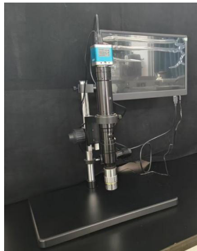
Figure 3. Microscopic photography system
