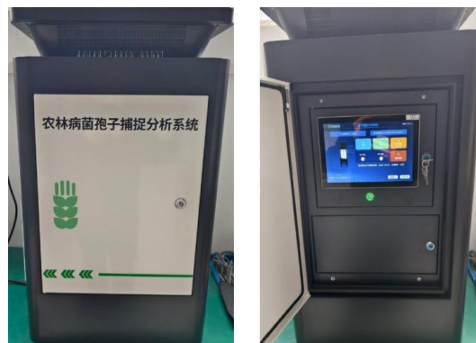
Figure 8. Wheat straw rust analyzer
