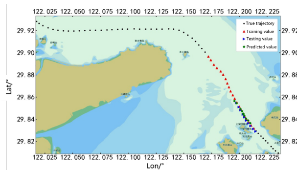
Figure 3. Trajectory prediction by the transformer model result diagram on an electronic nautical chart
