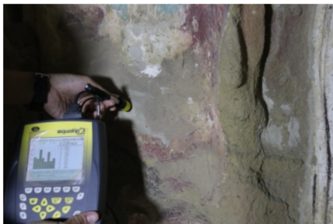
Figure 2. Testing the surface hardness of rock with a portable Leeb hardness tester
