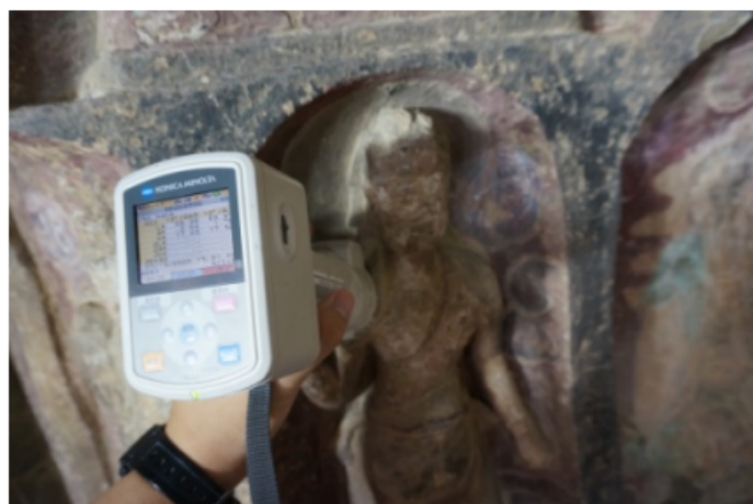
Figure 3. Detecting the color of the polychrome surface with a spectrophotometer
