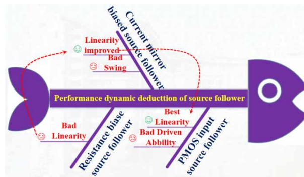
Figure 2. “Performance elements dynamic deduction” of the source follower.
