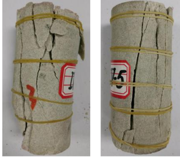
Figure 3. Splitting failure mode of specimen.
