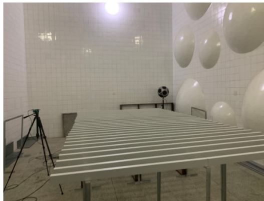
Figure 4. Reverberation room method for sound absorption coefficient testing
