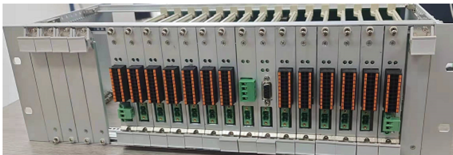
Figure 2. Appearance diagram of LED railway signal lamp filament alarm monitoring device
