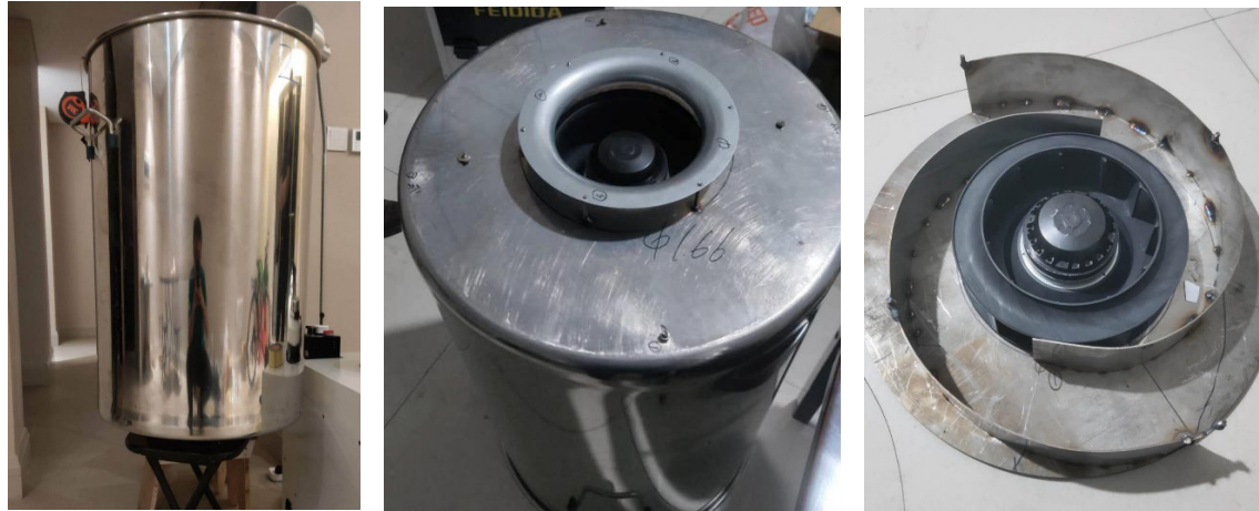
(a) tank(stainless steel barrel) (b) Bottom of the tank (c) blade and fan module
