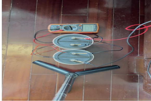
Figure 10. High-voltage capacitor constant current charging test.
