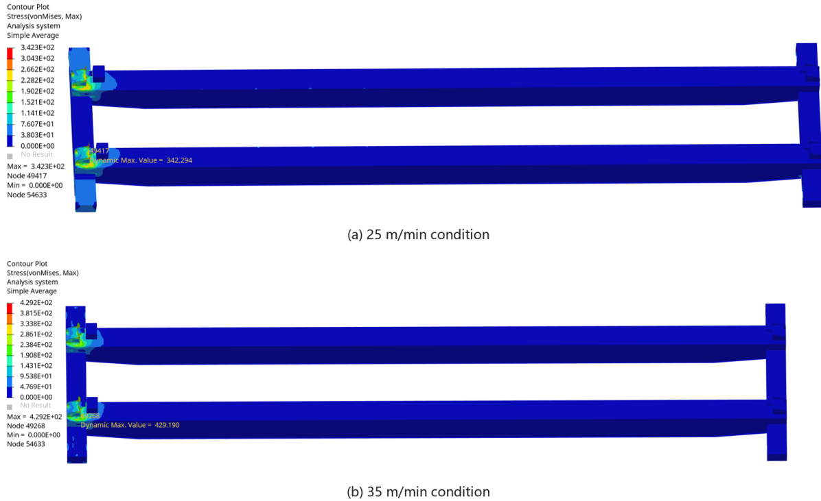
Figure 7. Global von Mises stress contours for both conditions.
