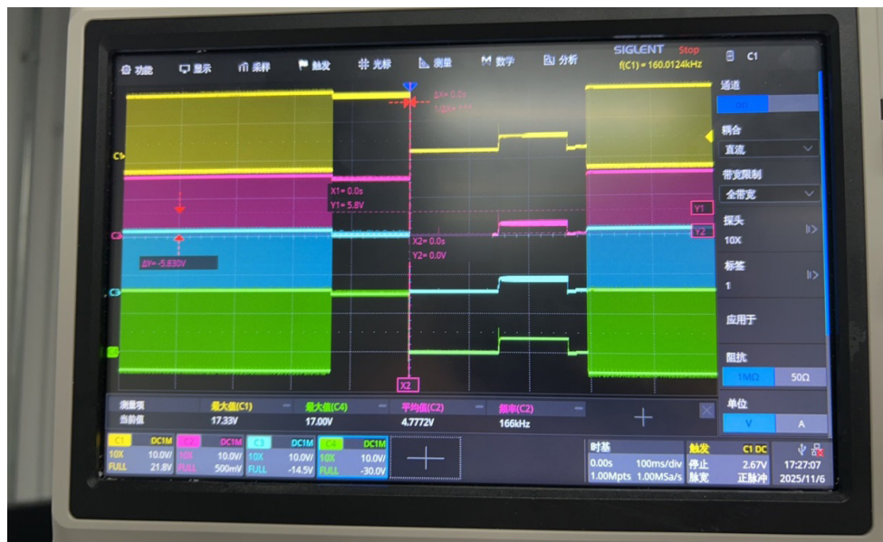
Figure 2. Threshold voltage test following positive bias after DGS completion.
