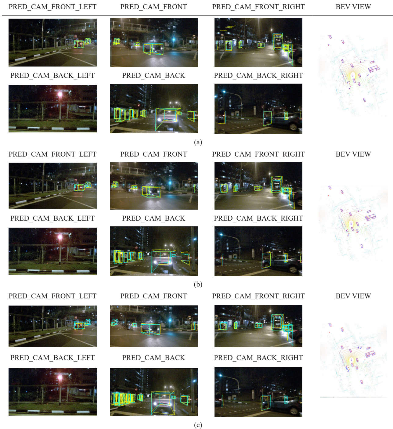
Figure 5. Qualitative comparison of detection results in a representative nighttime scene. In each subfigure, the left part shows six-camera-view detection results, where yellow boxes denote predictions and blue boxes denote ground truth. The right part shows the corresponding BEV visualization, where dark blue boxes denote predictions and red boxes denote ground truth. (a) Ours; (b) Zero-DCE; (c) SMG.
