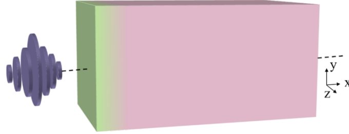
Figure 1. Combined acceleration model of RPA and LWFA driven by circular polarization laser. The green part represents a critical density thin target with a thickness of 5 \mu\text{m} , and the pink part represents an uniform density plasma channel.
