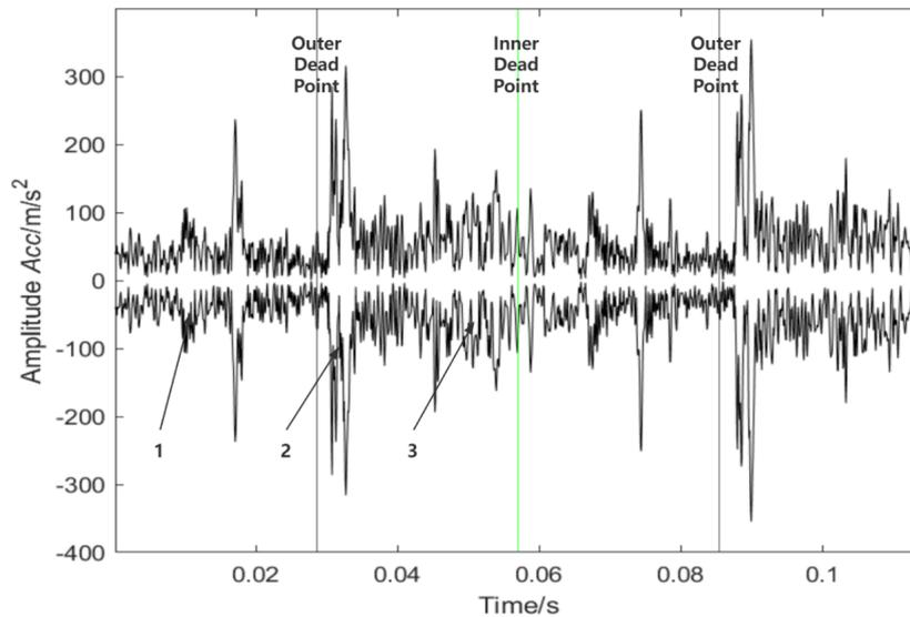
Figure 6. Vibration signal envelope diagram of Case 1.
