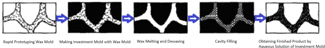
Figure 2. Process flow of porous aluminum production via the indirect method.
