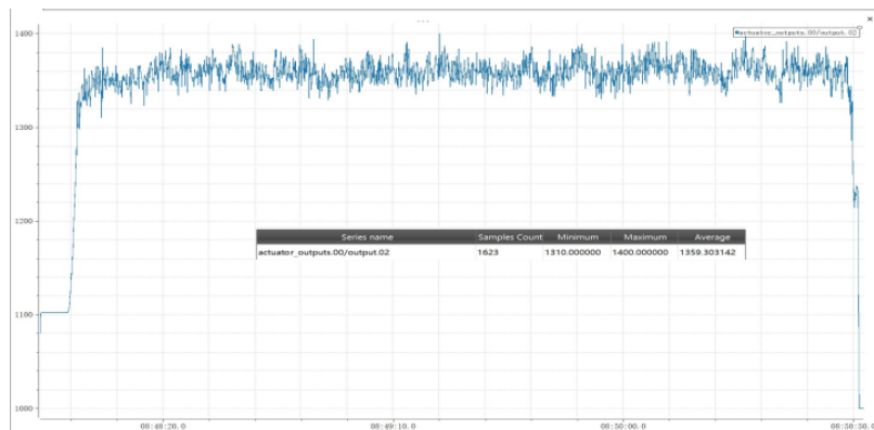
Figure 8. Throttle curve in position mode.
