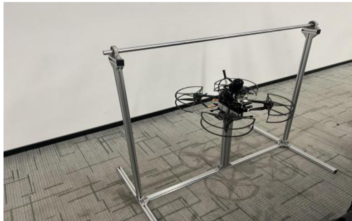
Figure 3. Attitude loop PID tuning.
