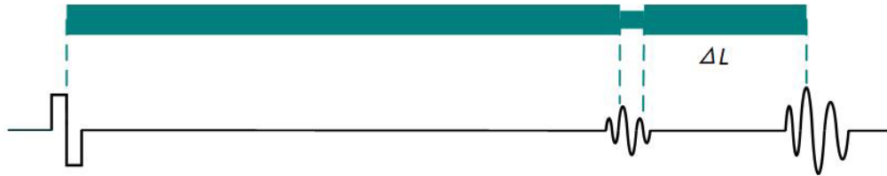
Figure 1. Principle of ultrasonic temperature measurement.
