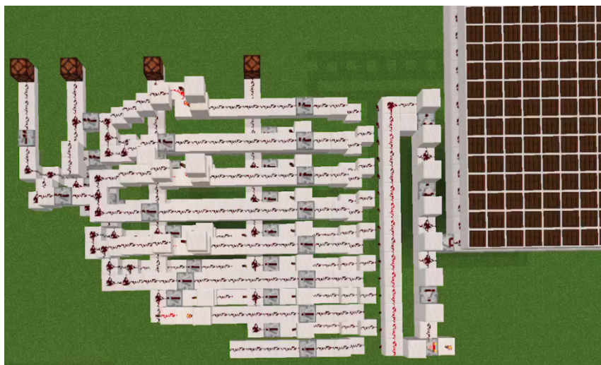
Figure 17. Realization of 1-bit hexadecimal to 4-bit binary number conversion circuit
