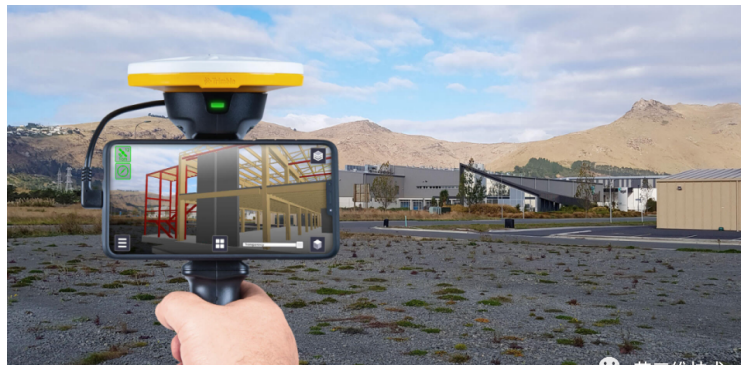
Figure 3. The MR technology superimposes the completed building renderings onto the actual construction site (*Web-sourced images)
