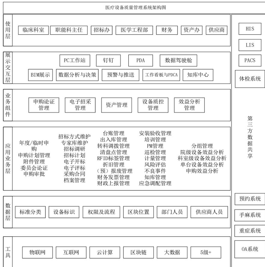
**Figure 1.** System architecture diagram (Abbreviations: PDA: Personal Digital Assistant; BIM: Building Information Modeling; RFID: Radio Frequency Identification; PM: Preventive Maintenance; HIS: Hospital Information System; LIS: Laboratory Information System; PACS: Picture Archiving and Communication Systems)
