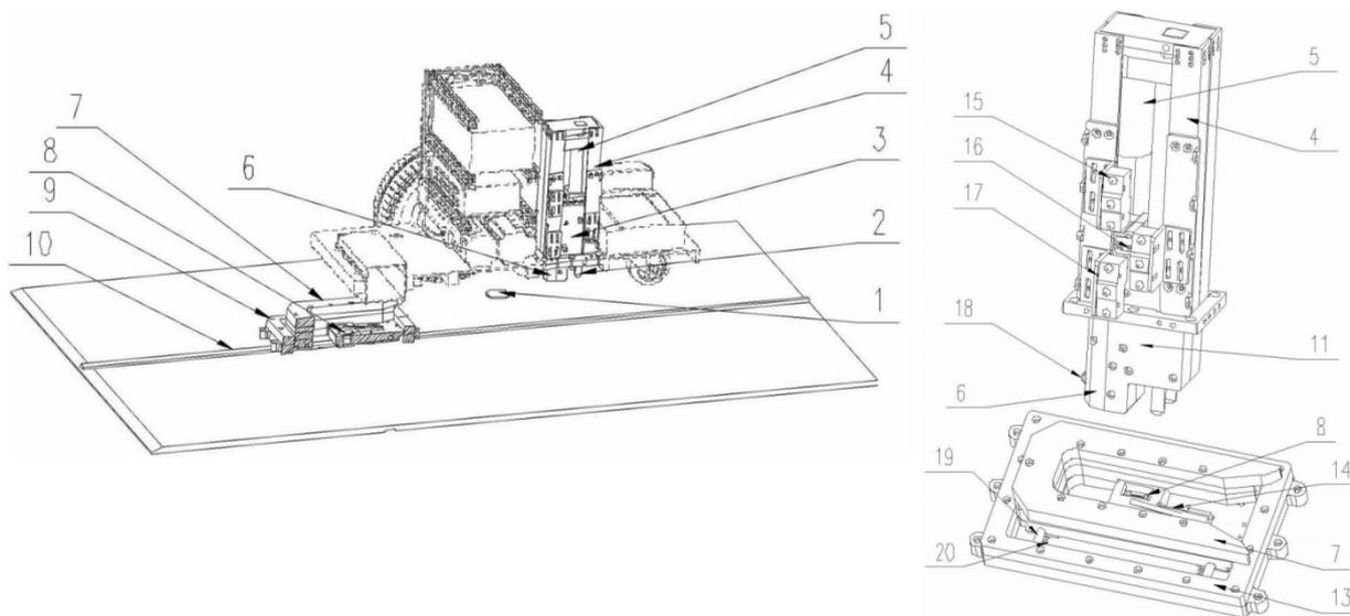
**Figure 3.** Left: Structure diagram of inspection robot; Right: Charging plug and charging socket structure diagram. Figure markings: 1, RF card; 2, copper plate; 3, plug body; 4, frame; 5, push rod motor; 6, inclined surface; 7, U-shaped guide plate; 8, socket; 9, base; 10, magnetic track; 11, plug; 12, fifth limit switch; 13, base; 14, limit switch; 15, first limit switch; 16, second limit switch; 17, third limit switch; 18, fourth limit switch; 19, guide rail; 20, spring.
