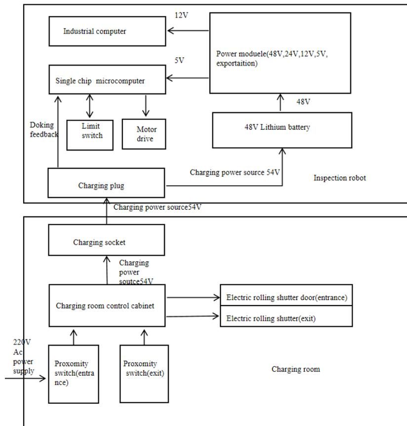
**Figure 1.** Block diagram of the automatic charging module
