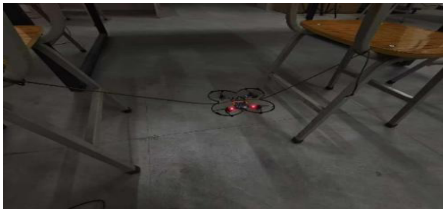
Figure 6. UAV Fuzzy PID control fixed axis test
