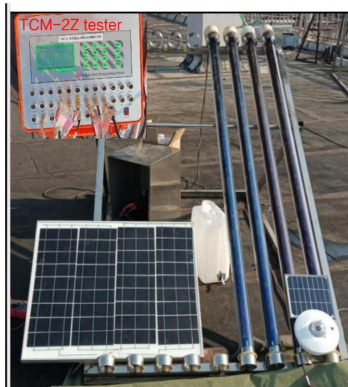
Figure 2. Physical setup of the solar-cooled PV/T system
