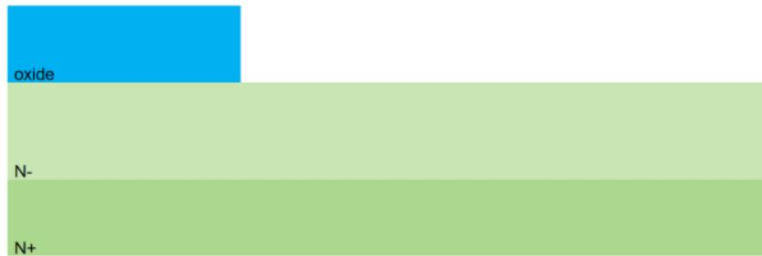
**Figure 4.** Schematic diagram of the isolation area
