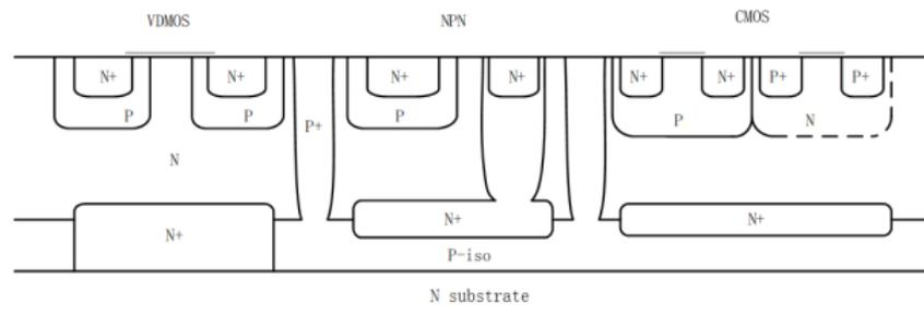
**Figure 1.** Schematic diagram of a power integrated circuit structure isolated by PN junction
