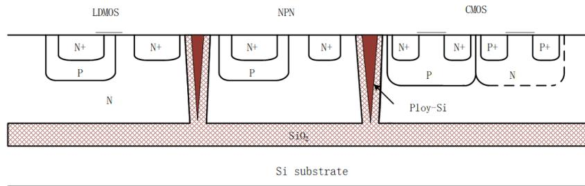
**Figure 2.** Schematic diagram of power integrated circuit structure with medium isolation
