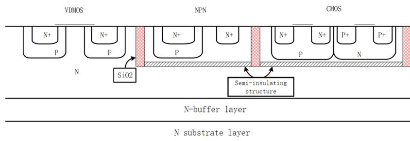
**Figure 3.** Schematic diagram of power integrated isolation structure
