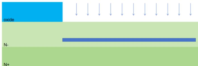
**Figure 5.** Schematic diagram of vanadium ion injection in the isolation zone
