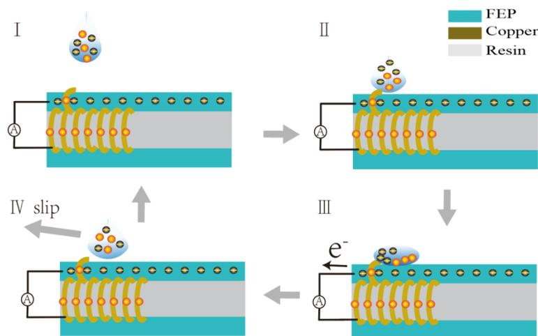
**Figure 1.** Schematic diagram of body effect power generation
