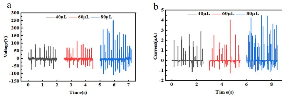
**Figure 5.** DEG output characteristics of different droplet sizes: (a) Output voltage diagram; (b) Output current diagram
