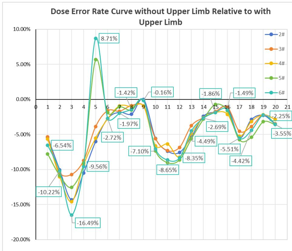
**Figure 3.** Dose error rate curve without upper limb relative to with upper limb. Note: The horizontal axis represents 20 sampling points on the phantom, and the vertical axis represents the dose error rate percentage. The curves show the dose error rates for collimators 2#, 3#, 4#, 5#, and 6# for irradiation without upper limb relative to with upper limb
