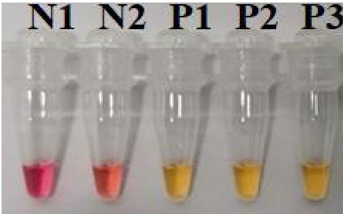
Figure 3. Colourimetric detection of RT-LAMP products.
