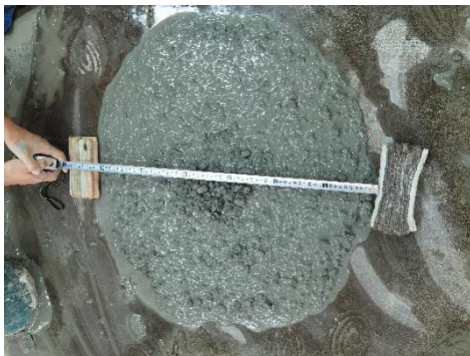
(a) Slump expansion test with strength of 60 MPa
