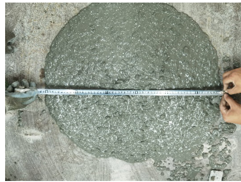
(b) Slump expansion test with strength of 80 MPa
