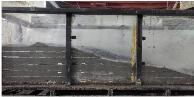
(b) Side view of tailings dam failure
