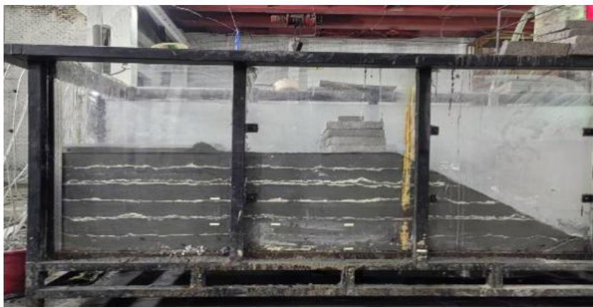
Figure 1. Schematic of lime layering and loading process.
