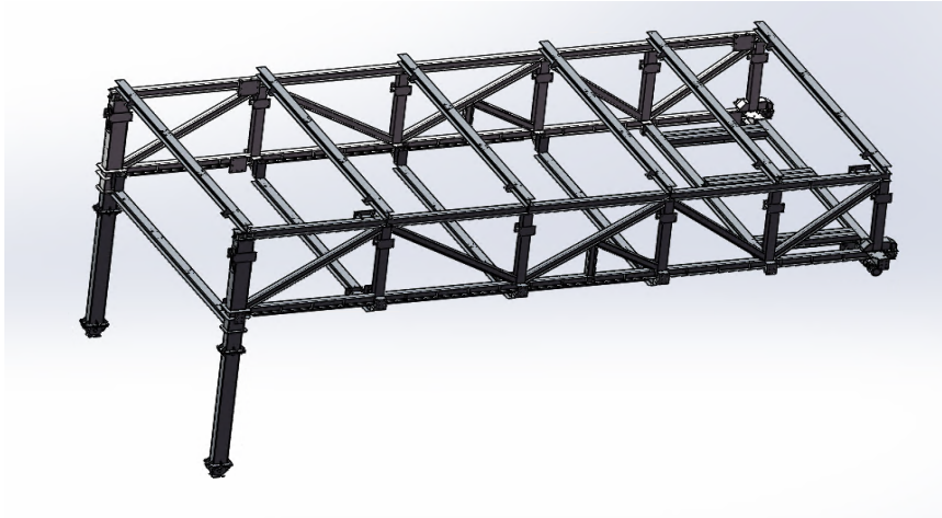
Figure 3. Schematic diagram of movable arch frame
