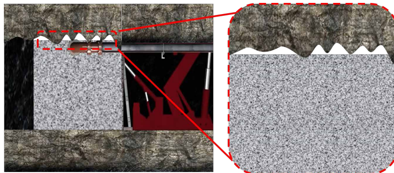
Figure 2. Gaps occurring in paste backfill roof contact
