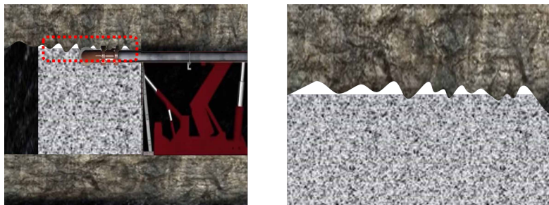
Figure 19. Diagram of paste backfill material failing to reach the roof
