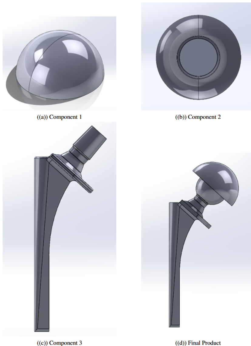
Figure 8. SolidWorks modeling of the femur showing individual components and the final assembled product
